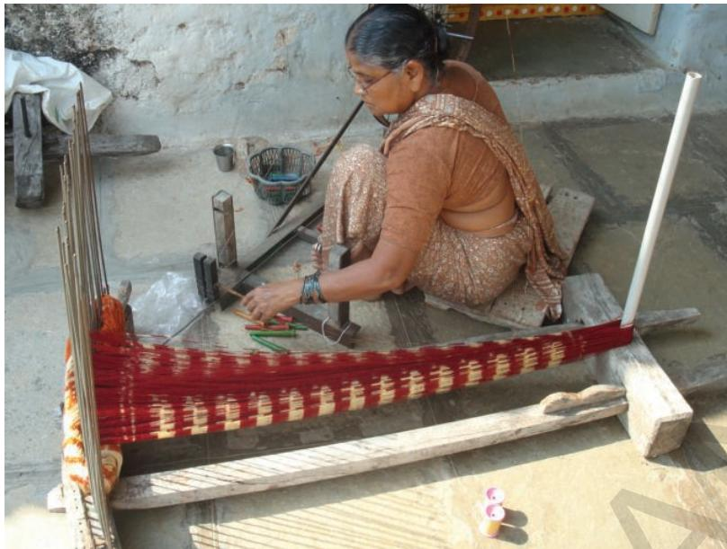
Fig 7.6 Bobbin winding
